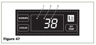
To display actual temperature in the refrigerator, press the "WARMER" button momentarily. A solid status indicator light (1, **Figure 47**) will show and the air temperature reading in the cabinet will show for approximately 10 seconds.
